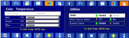
Push "Left" or "Right" to select Color Temp between Push "Up" or "Down" button to select between "Default", "System 1", "System 2", "System 3", or "DPMS", "Auto Source Select", or "Freeze Frame" "System 4" then push "Select" then push "Select" Use "Left" or "Right" button to
